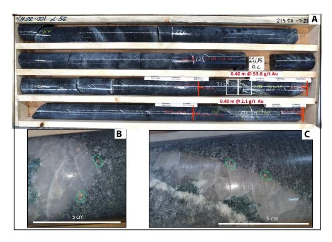
Figure 6. Core Photo from VM22-001, showing visible gold on quartz vein contact (green circles on zoom in photo B and C below). The intercept returned 53.8 g/t gold over 0.40 m (ETW 0.20 m).
