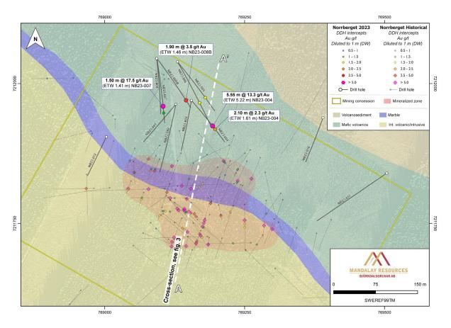
Figure 2: Plan view showing 2023 drilling in relation to historic intercepts and previously identified mineralisation. Composited intercepts that, when diluted to 1m, grade above 2g/t are annotated.
