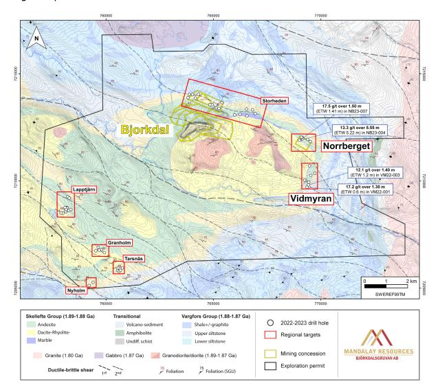
Figure 1. Geological Map centred on Mandalay exploration tenement holdings highlighting the location of exploration drilling described in this release. Highlighted assays results are annotated.
