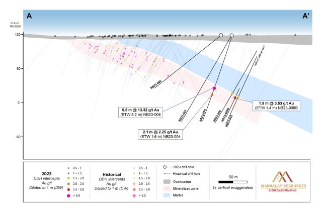
Figure 3 Cross-Section of the Norrberget orebody showing recent drilling. See figure 9 for location. Composited intercepts that, when diluted to 1m, grade above 2g/t are annotated.
