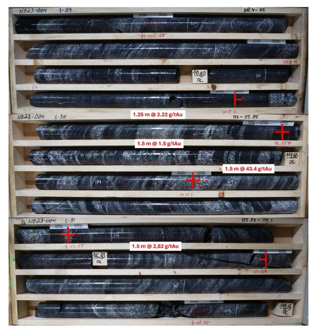
Figure 4: Picture of NB23-004 drill core through the of the orebody showing mineralisation and individual assays grades. The combined interval was 13.3 g/t gold over 5.55 m (ETW 5.22m).
