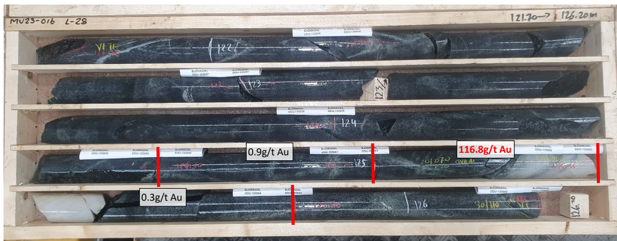
Figure 3. Photograph of core from MU23-016 (125.00m – 125.35m – ETW 0.27m @ 116.8 g/t Au).
