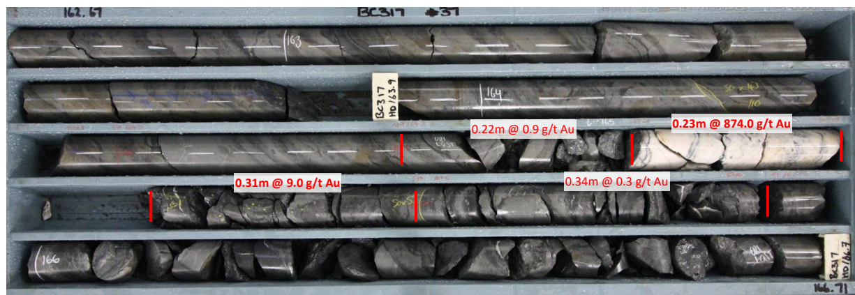
Figure 1. BC317 Core tray showing gold bearing quartz veining representative of the northern portion of the Suffolk vein.
