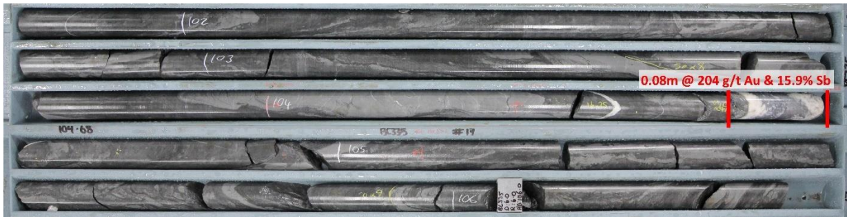
Figure 3. BC335 Core tray showing quartz-stibnite veining representative of the southern portion of the Suffolk vein.
