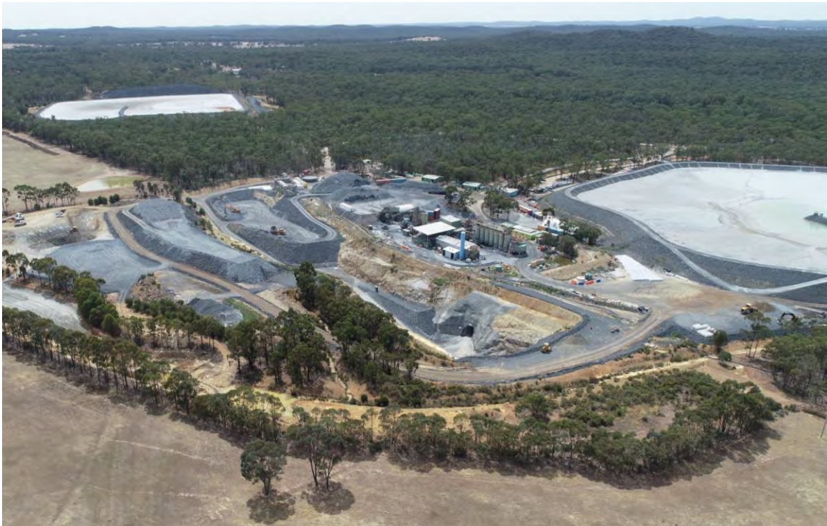
Figure 5-3: Aerial View of the Brunswick Complex with Brunswick Portal (middle of image), Brunswick Processing Plant, offices and tailing storage facilities.
