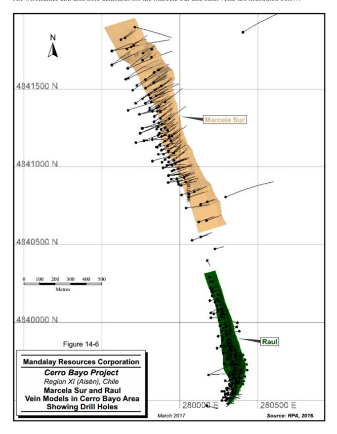
The Au and Ag grades were estimated using an anisotropic Inverse Distance Cubed model and were validated by several methods, including visual inspection and statistical comparisons with composite assay statistics and wireframed volumes. Domain models were used as hard boundaries to limit the extent of influence of composite grades within the domains.
